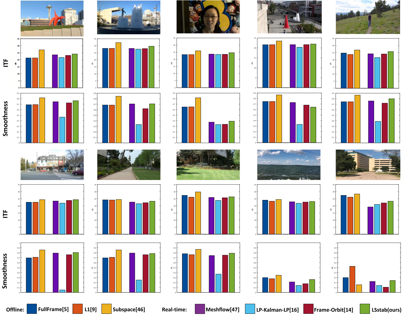
Fig. 11. Comparison with state-of-the-art video stabilization algorithms. Higher ITF and Smoothness means better stabilization result.
